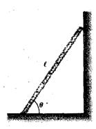
A uniform ladder of length l and weight rests against a smooth, vertical wall as shown in the figure. If the coefficient of static friction  $\mu_s$  between ladder and the ground is 0.40, calculate the minimum angle  $\theta_{\min}$  at which the ladder does not slip.
