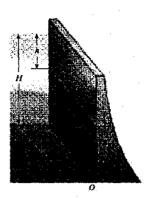
Water having a density  $\rho$  is filled to a height H behind a dam of width w as shown in the figure. Determine the resultant force exerted by the water on the dam. (Here g is the acceleration due to gravity.)
